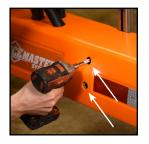
**10)** Once the boom is secure, tighten the hardware on the boom brackets to make sure they are also secure.
