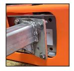
**6)** If you are using the boom brackets to mount the boom to the applicator, insert the bolts through the bracket and place plastic washers over bolts to hold them in place.
