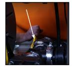
3) Place the 3-way valve in recirculation position to allow liquid to recirculate back to the tank. If your applicator is GPS flow controlled, you will need to manually open the electric flow control valve using your Storm Commander® controller (refer to your Storm Commander® "Operating" instructions).
