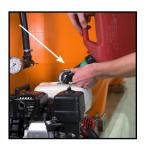
**17)** If you have a gas powered unit you will also need to remove the oil cap and fill the engine with 0.61 US quarts of 10W-30 engine oil.
